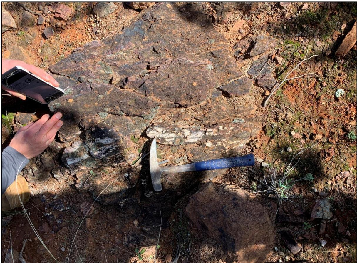
**Figure 7** Rockchip sample location RARK004 prior to sampling showing gossanous brown rock and white quartz veins, hosted in foliated ex-sulphide bearing sediments and near the eastern contact with coherent rhyolite (out of picture).
