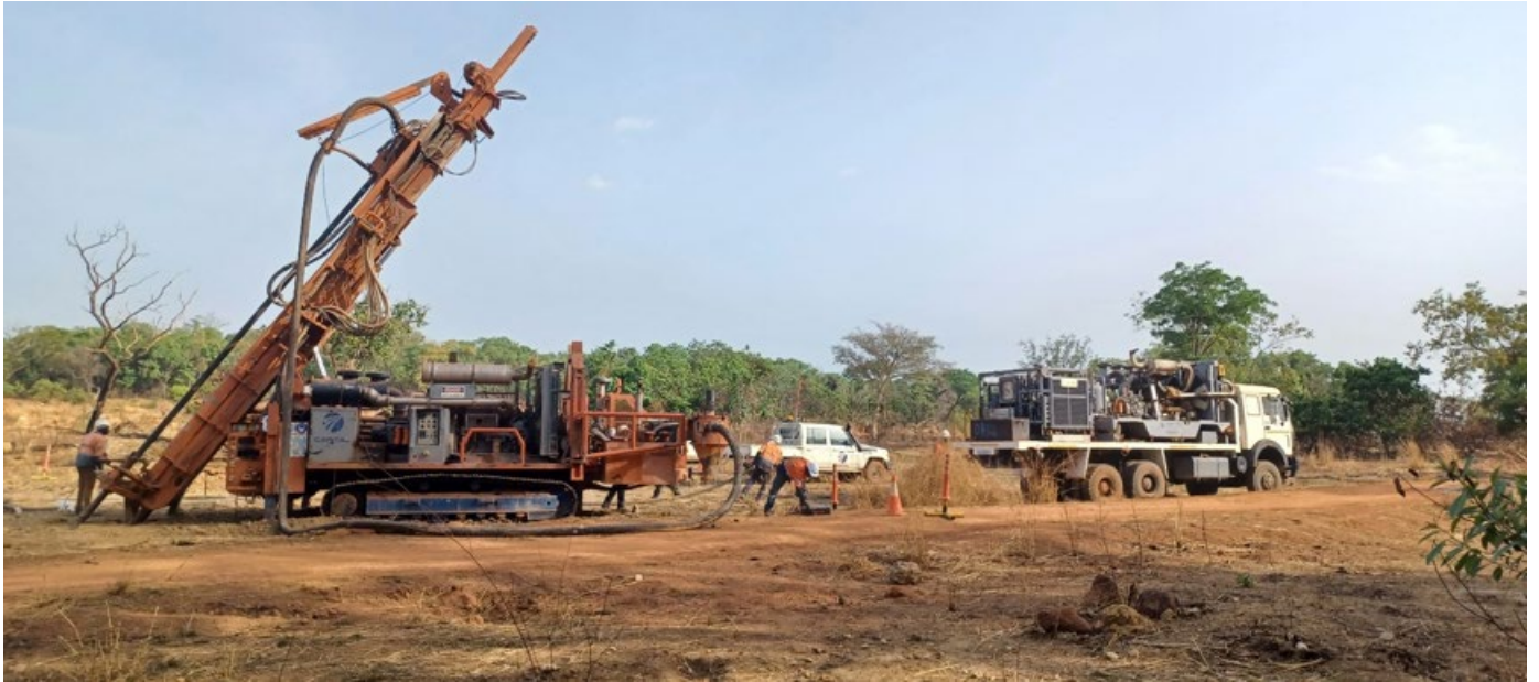
Figure 3: RC drilling at 800W
