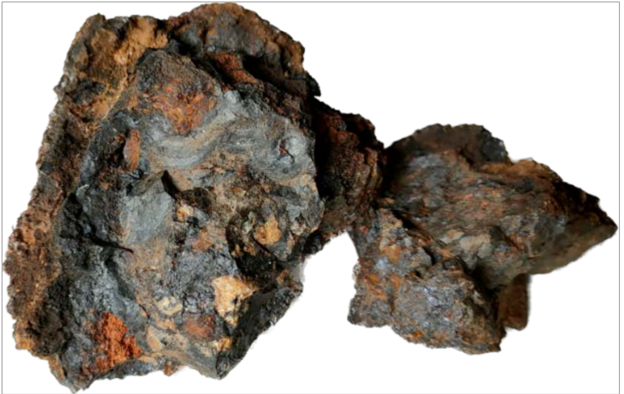
Figure 4: Sample (CD23_035) of manganiferous gossan from the North Gossan that is elevated in copper, cobalt, barium and nickel.
