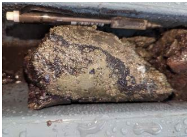
Chalcopyrite hematite lode in replaced ultramafic at 403.9m.
