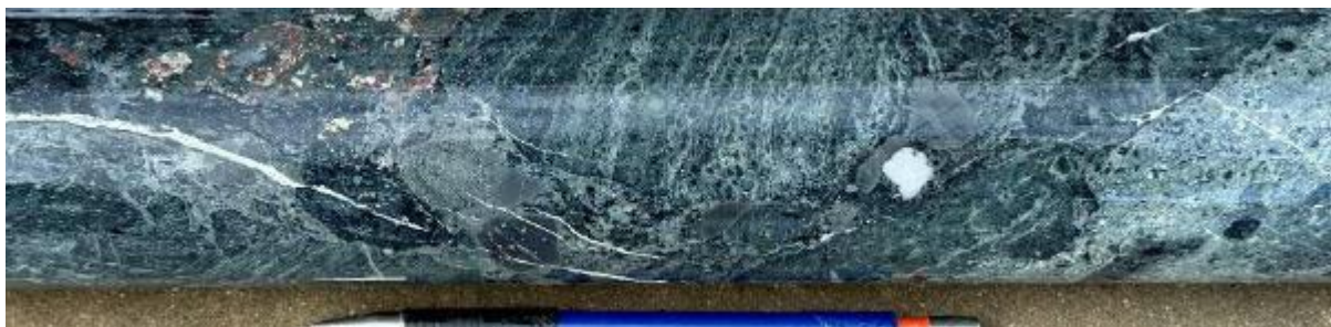
Polymictic breccia with juvenile flow-banded diorite clast, quartz vein clast and mineralised clasts. 607.7m.
