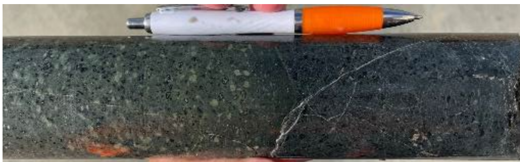
Chilled margin with LKD at contact with chlorite-altered, mineralised microdiorite at 456.2m.
