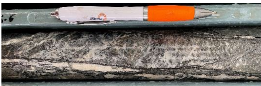
Fractured diorite with carbonate infill at 692.5m.
