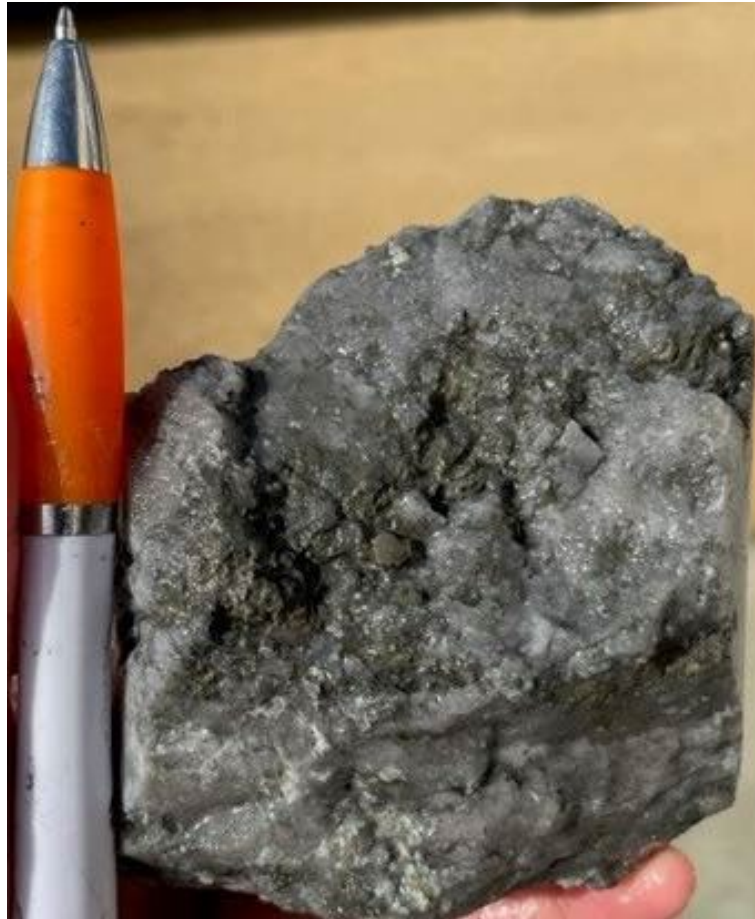
Part of 20cm Quartz-pyrite vein with trace supergene chalcocite and chalcopyrite within microdiorite at 162.5m.
