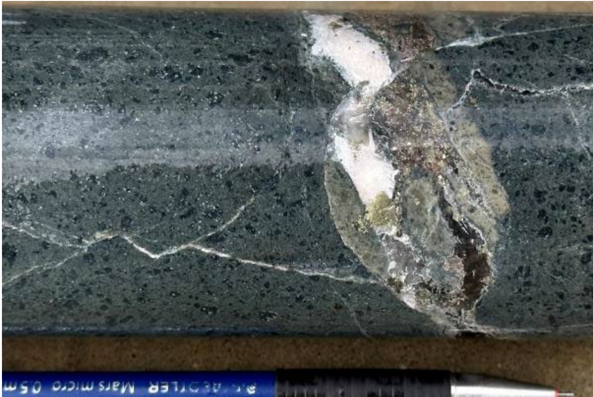
Complex pyrite+chalcopryite+hematite+gypsum+carbonate vein. 604.9m.
