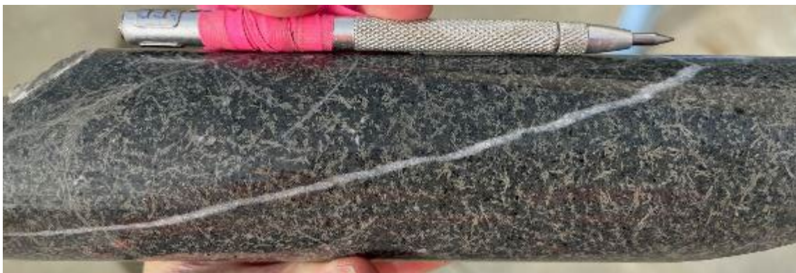
Sericite/chlorite after Actinolite, probably rutile (bladed texture) in fine-grained diorite at 751.8m.
