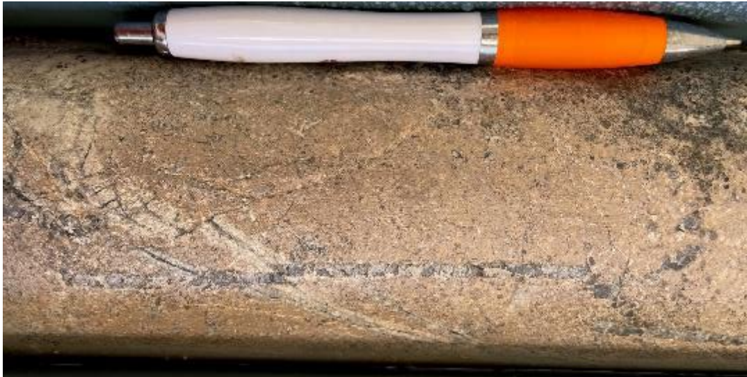
Buff coloured, clay altered microdiorite with quartz-pyrite-supergene chalcocite veins at 51m.
