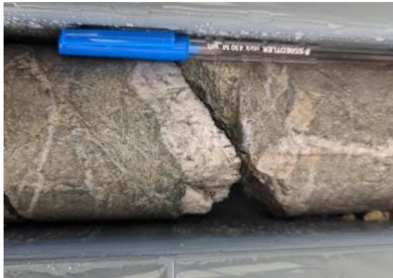
Microdiorite with quartz A veins at 275m.
