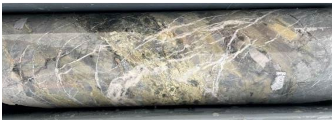
Brecciated Siltstone with strong sericite alteration and blebs of pyrite overprinted by quartz-carbonate stringer veins at 380.4m.
