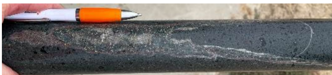
Quartz-carbonate-hematite-pyrite vein in chlorite altered diorite at 703m.
