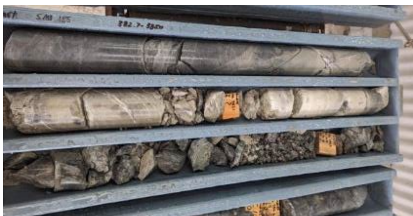
Carbonate shear LAS? at 382m.
