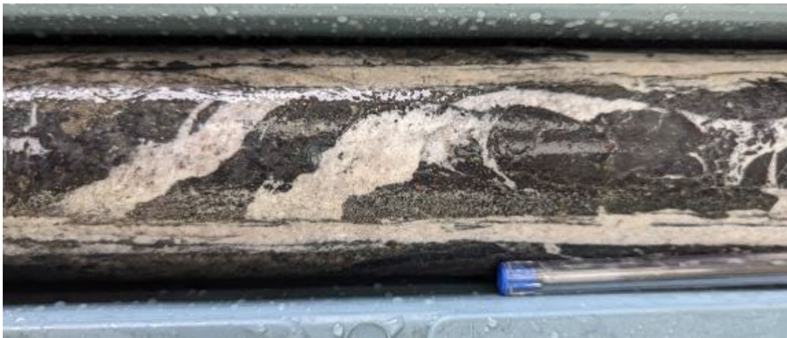
Quartz carbonate ladder vein at 647m.
