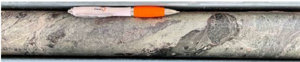
Talc-dolomite altered serpentinite at 483.9m.
