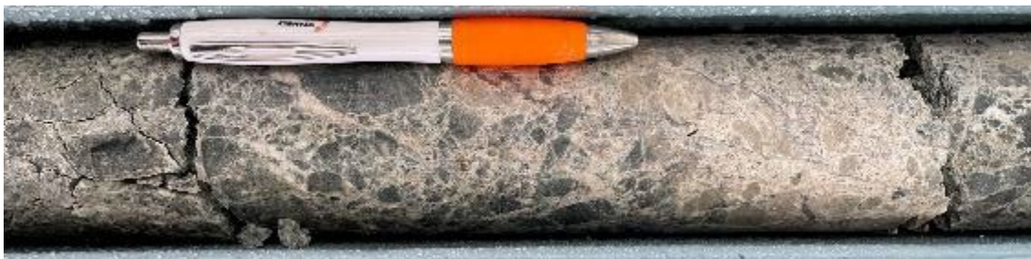
Fractured Microdiorite with clay infill at 525m.
