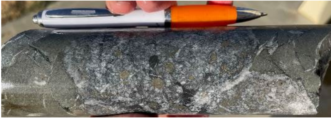
Low temperature brecciated quartz-carbonate vein with blebs of pyrite in andesite at 823m.
