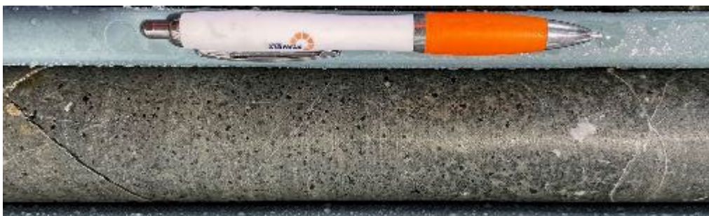
Andesite/diorite at 786.2 showing 1-2mm sized mafic phenocrysts.
