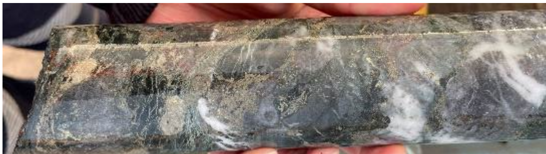
Complex quartz vein with magnetite-hematite-pyrite-chalcopryite in mudstone at 735.5m.
