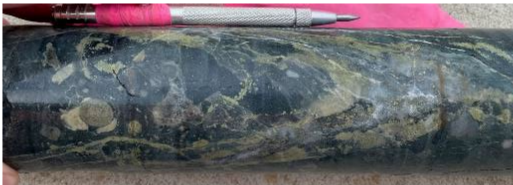
Quartz-chalcopyrite-pyrite vein with epidote selvage in chlorite altered Alfa Breccia at 421.2m.
