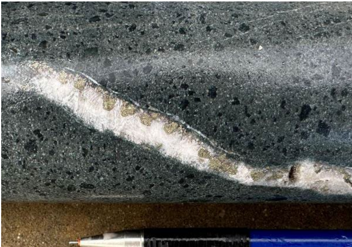
Pyrite+chalcopryite vein that has been re-opened and filled with carbonate+quartz. 606.4m.
