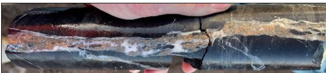
Photo 1. Quartz-carbonate-sphalerite vein in mudstone at 775.9m.
