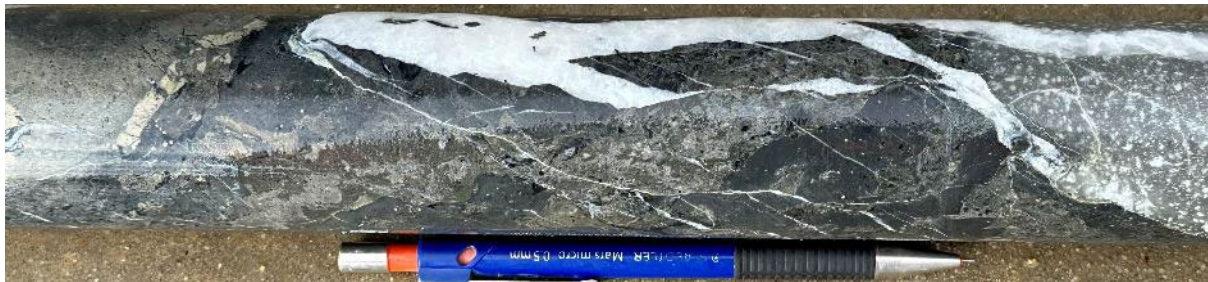
Contact between polymictic breccia and diorite cut by a late quartz+carbonate vein. 878.0m.
