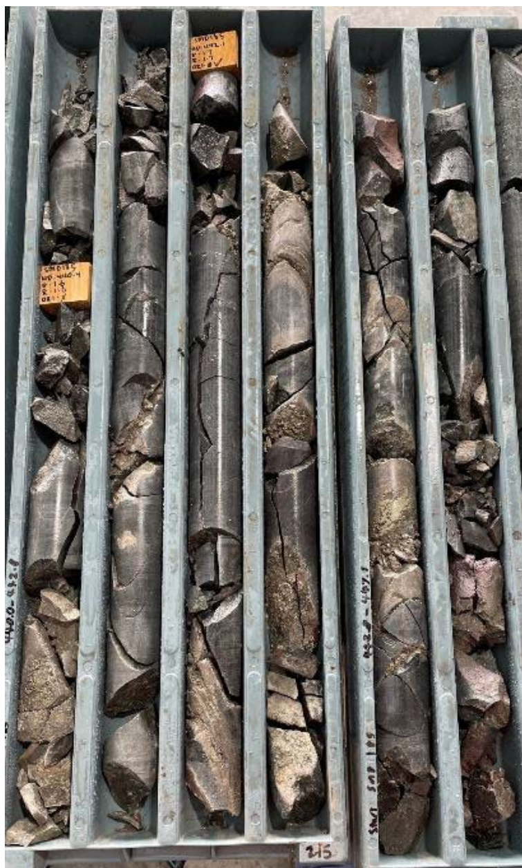
Zone of increased (10%) quartz-hematite-chalcopyrite-pyrite veins in Alfa Breccia at 440-444m.
