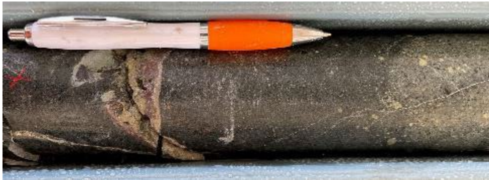
Quartz-hematite-chalcopyrite vein with chlorite selvage in microdiorite at 483.9m.
