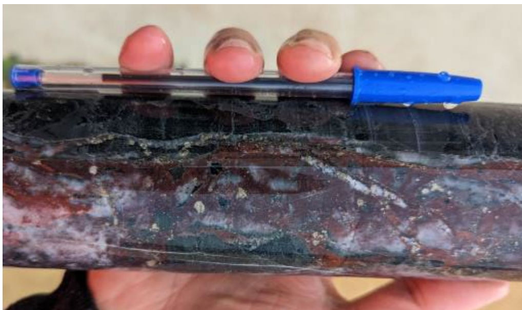
Quartz carbonate ladder vein at 647m.
