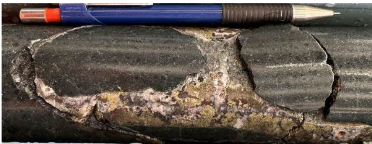
Chalcopyrite+pyrite+quartz+carbonate vein. 613.15m.
