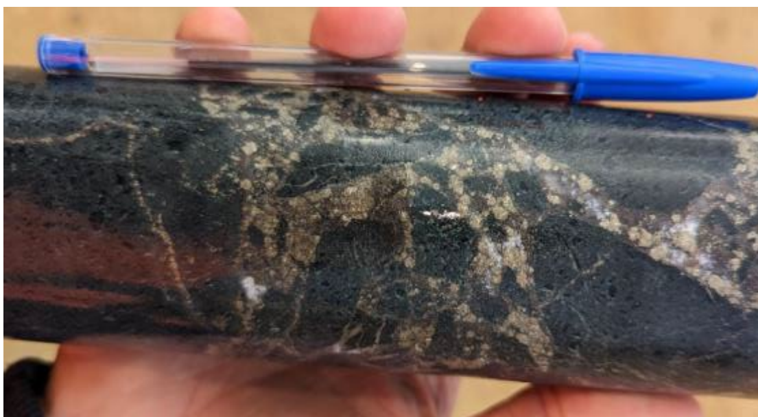
Quartz hematite pyrite chalcopyrite crackle breccia vein at 679m.
