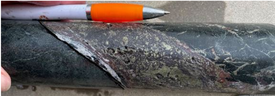
Quartz-hematite-magnetite-pyrite-chalcopryite vein on diorite/mudstone contact at 729.4m.
