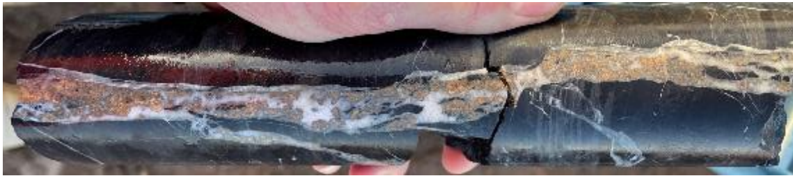
Quartz-carbonate-sphalerite vein in mudstone at 775.9m.
