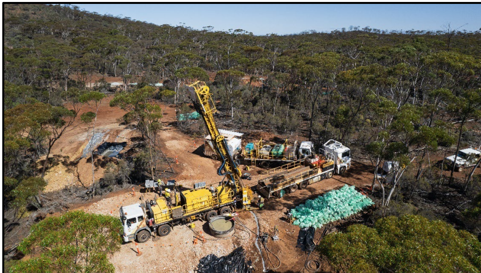
Figure 1 — Diamond drilling on site at Galileo's 100% owned Callisto discovery near Norseman.
