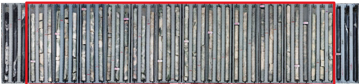
Figure 3: Drill hole SADD077: 33.05m @ 1.83% Li 2 O from 319.53m. Refer to ASX announcement dated 23 March 2023
