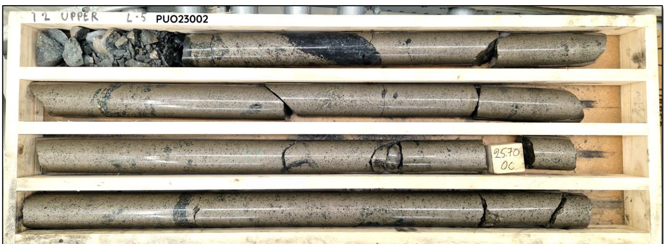
Figure 1: Massive sulphide (pyrrhotite-chalcopyrite) from drillhole PUO23002, approx. depth 24.2-26.9m downhole.
