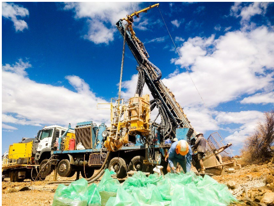
Plate 1 – RC drilling - Northern Apollo Hill (late February 2023).
