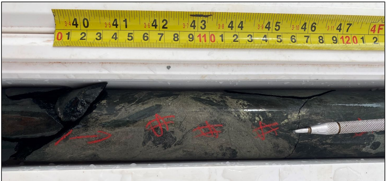
Figure 5: Massive/stringer sulphides in DKDD0035 at 501.8m
