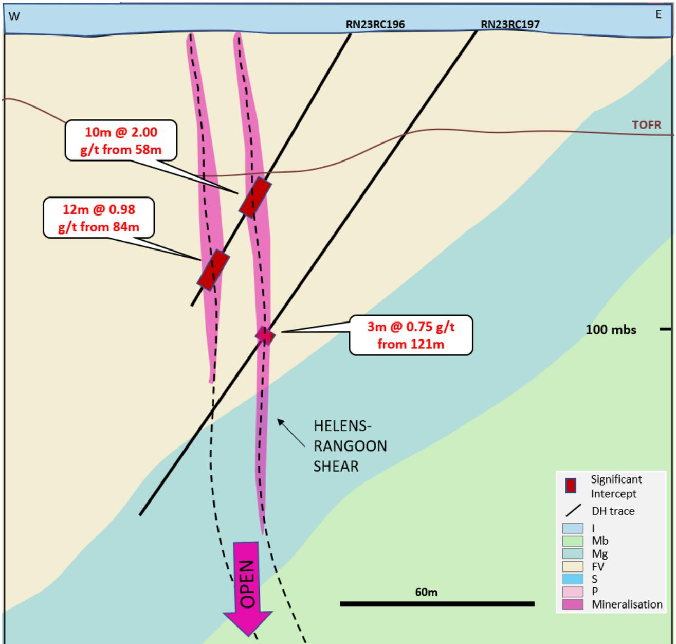
Figure 4 – Schematic Cross-Section through A-A' looking north on 6815600N showing recent drilling with reported intercepts. Interpreted mineralised structures shown in pink. True width is approximately 70% of down-hole width.
