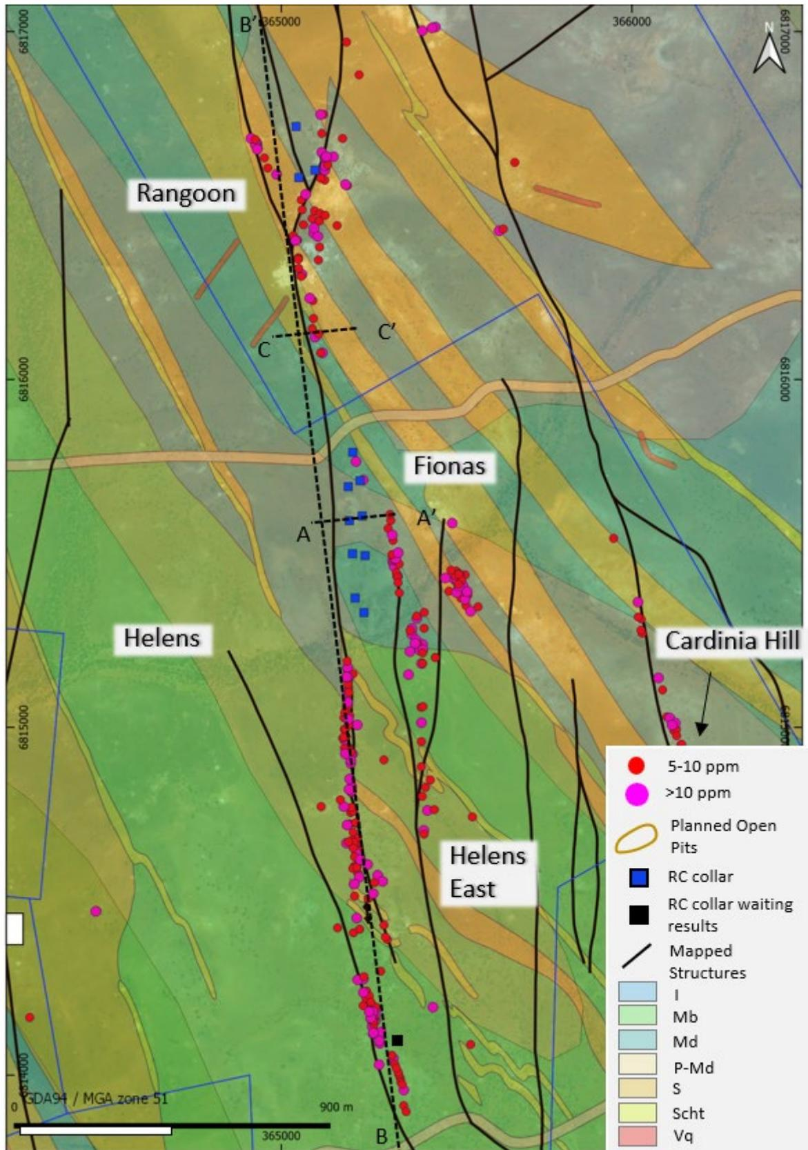
Figure 2 – Geological Plan of the Helens-Rangoon RC holes, showing collar positions relative to the +5.0 and +10.0g/t Au down-hole intersections for previous drilling, overlain on the mapped geology and structure. Cross section A-A' and C-C' location shown in Figure 4, Figure 5 and long section B-B' in Figure 6.
