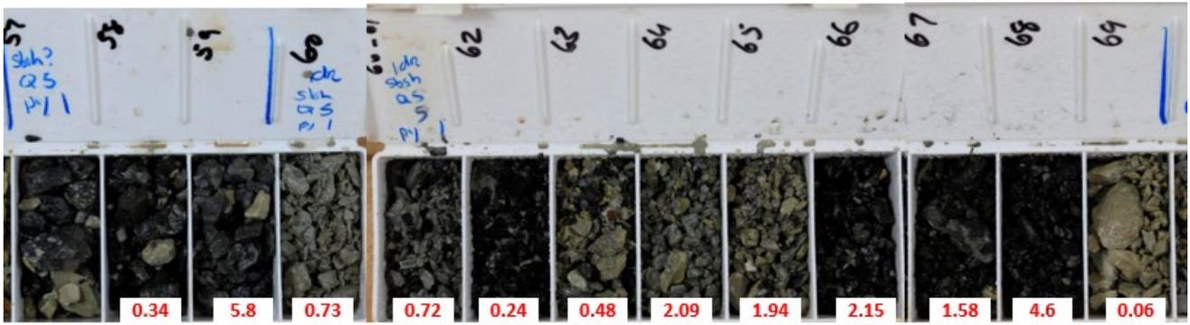
Figure 3 – Chip tray photo of mineralised intercept in RN23RC196, 59-69m down-hole showing logged sulphide content (blue numbers) with moderate quartz veining and gold assay results in g/t (red numbers).
