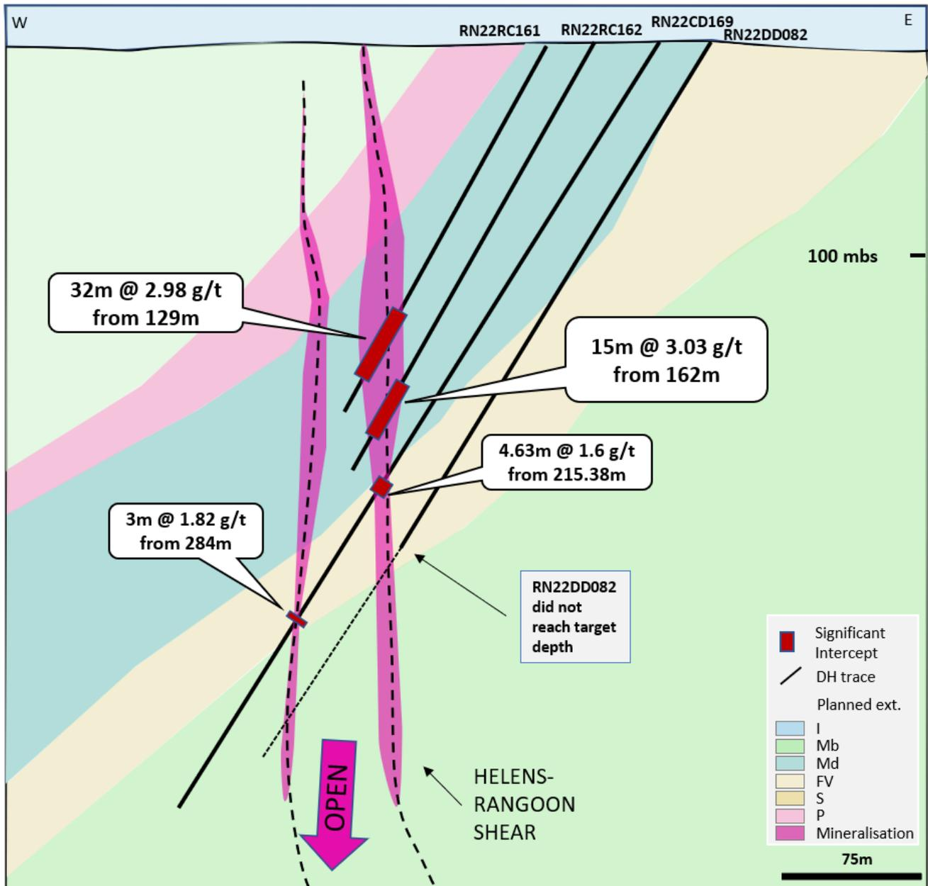
Figure 5 – Schematic Cross-Section through C-C' looking north on 6816100N showing two mineralised structures at the southern end of Rangoon, interpreted to be part of the larger Helens-Rangoon shear. Results are from announcements 27/6/2022 and 13/12/2022. True width is approximately 70% of down-hole width.
