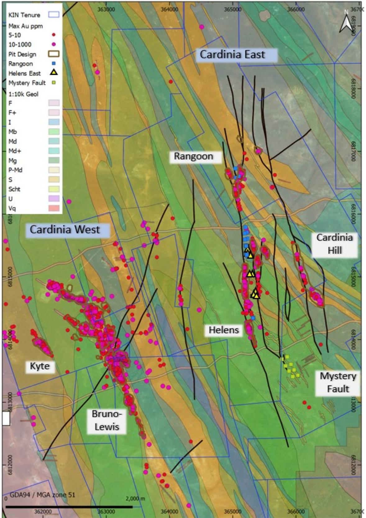
Figure 1. Plan view of Cardinia Gold Project showing the West and East mineralised corridors with extensive high-grade drill-hole (+5.0g/t and +10.0g/t Au only) trends along fault positions. Recent RC drill-hole collars at the Helens-Rangoon Fault target are shown.
