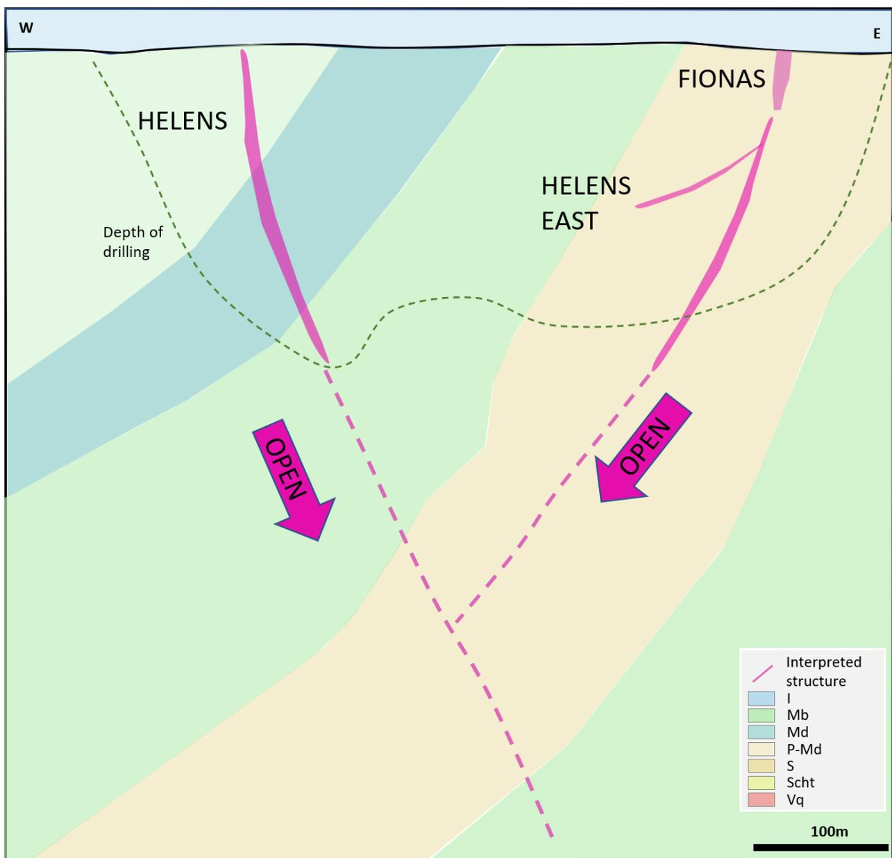
Figure 7 – Schematic Cross-Section looking north through the Helens – Helens East deposits, showing the interpreted interaction at depth. There is no drilling information below 200m.
