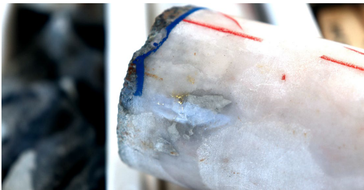
Figure 1: Visible gold 1 in PGRD23101 (~52m depth). Assays are pending for this interval.
