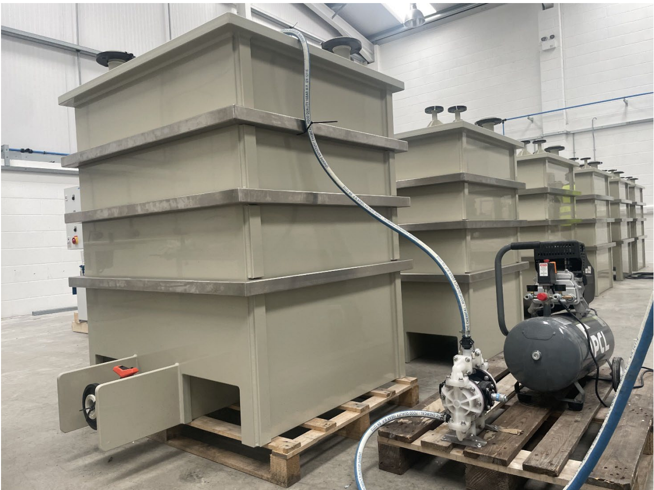
Figure 1: Process reactors undergoing hydrostatic testing.
