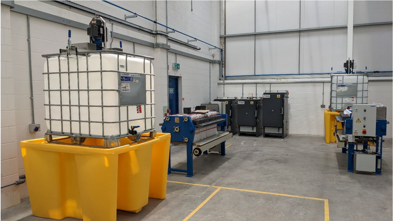
Figure 4: Plate and Frame filters in position along with process vessels and product drying kilns.
