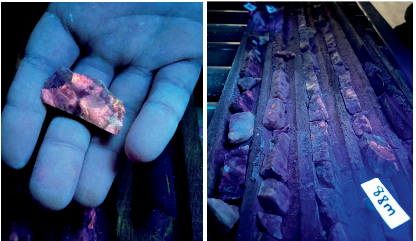
Figure 1 Photos of samples from XL-22 with visible Spodumene present under UV light, typically as 3-5cm crystals from interval grading 15.12m @ 1.4% Li 2 O from 73.6m.
