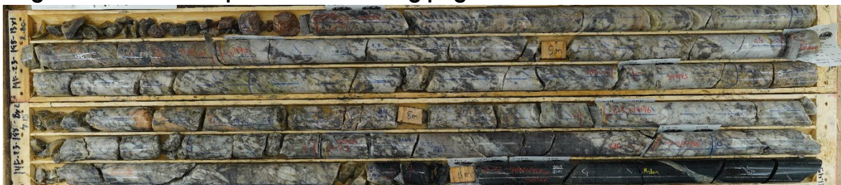
Figure 2 – MF23-198 Spodumene-bearing pegmatite from 3.1m to 7.65m down hole
