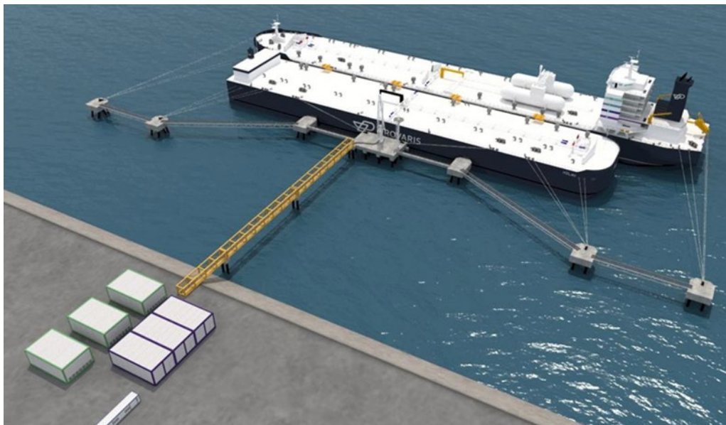
Figure 2: Illustration of the H2Leo Floating Storage integrated with H2Neo 430t carrier for loading/unloading
