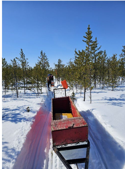
Figure 3 – Stepwise Moving Loop Transient Electromagnetic Survey, SQUID Sensor
