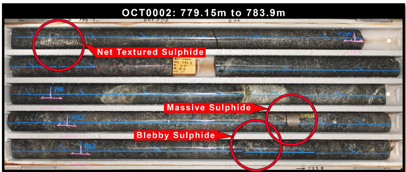
Photo 1: Diamond drill core tray from OCT0002 with visual Ni-Cu sulphide mineralisation, proximal to Target area B.
