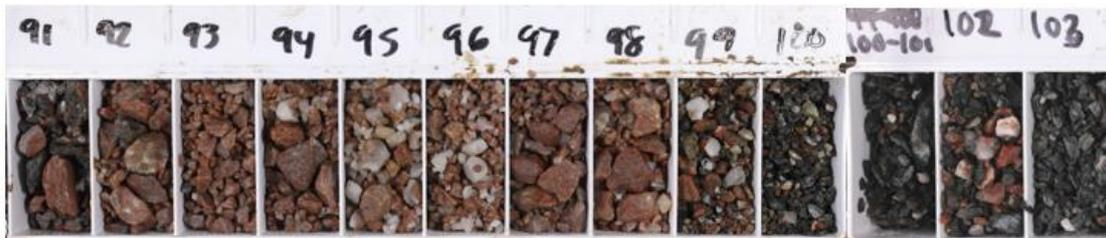
Photo 1: NMWBRC22-605 90-103m – Hematite + Albite + Quartz altered Quartz Porphyry (10m @ 5.80g/t Au - within 13m @ 4.53g/t Au from 90m)
