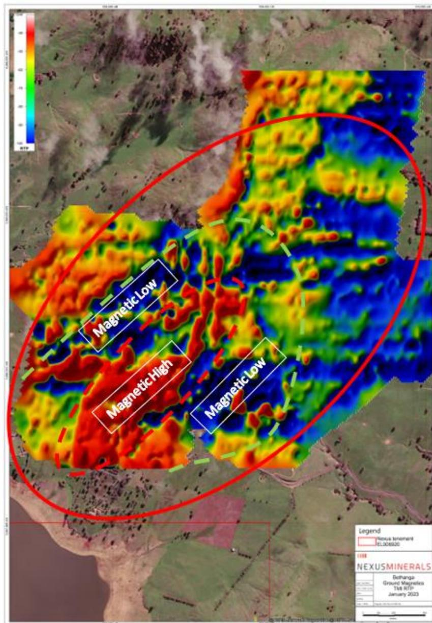
**Figure 11: Detailed Ground Magnetics Image (TMI RTP) over Aeromagnetic Anomaly (Anomalous area 3km x 1.5km highlighted with red outline – same area as highlighted in figure 10)**
