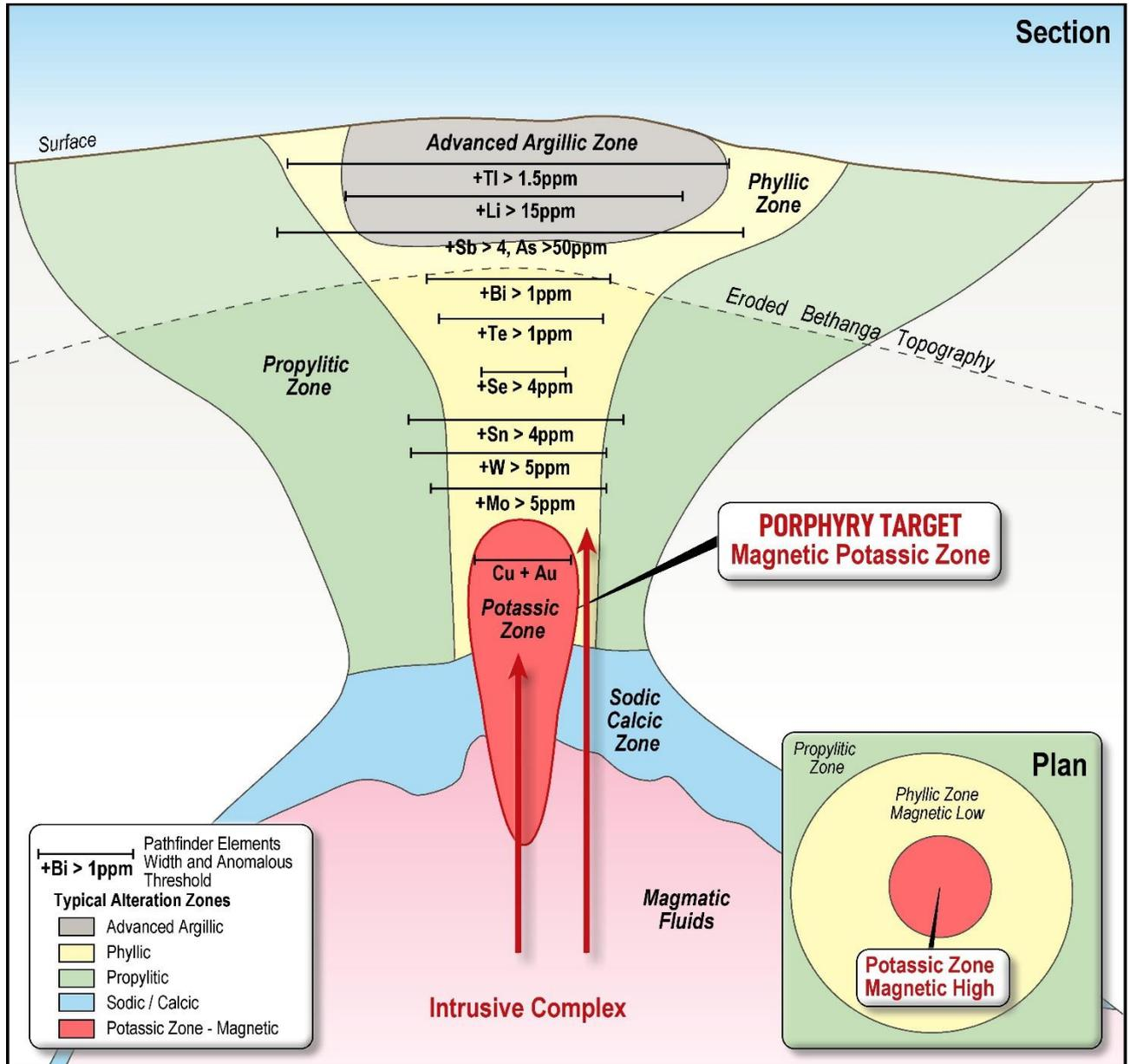
**Figure 9: Schematic diagram showing the geophysical signatures of the potassic and phyllic zones. Also the pathfinder geochemical and alteration patterns of a typical porphyry CU-Au mineral system (modified from Halley et al .,2015)**
