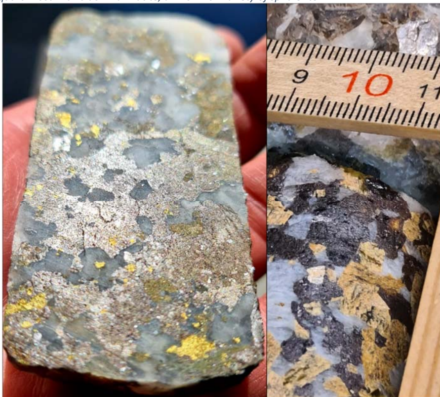
Figure 6. Left image: Half-core (width approximately 40mm) showing marmatite, sphalerite and chalcopryite from the lower zinc-copper zone (86.2 to 89.9m) . Right image: Drill core interval showing coarse grained siderite and marmatite in a quartz host.
