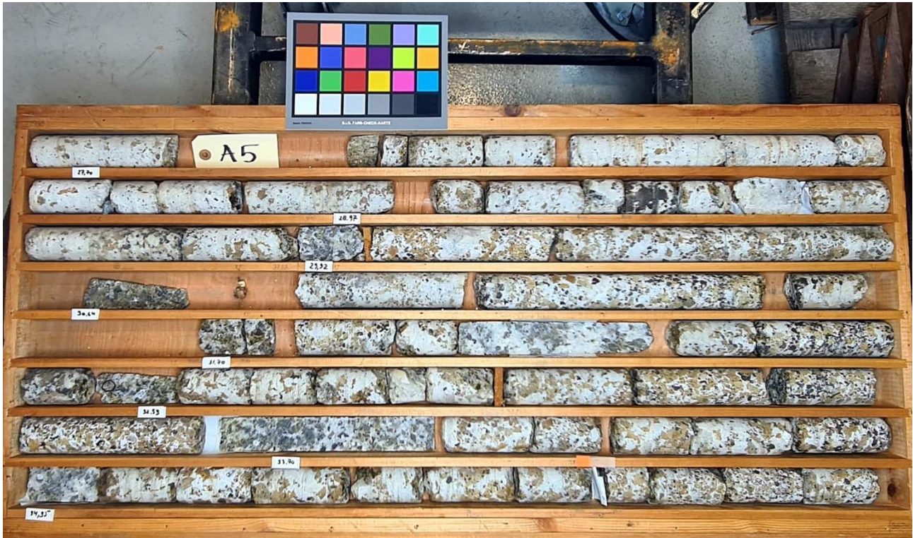
Figure 5. Diamond drill core from Hole A, upper zinc zone (approximately 26.8 to 35.2m down hole), showing siderite and sphalerite mineralisation in a quartz host with black marmatite, an iron-rich variety of sphalerite.
