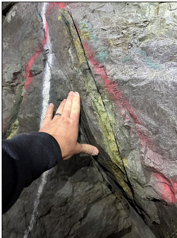
Photo 2 – Channel cut undertaken as part of underground sampling program. Note massive chalcopyrite mineralisation in the cut.
