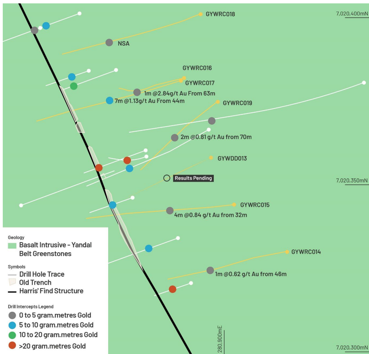
Figure 13: Plan section of reported drill-hole results positions.
