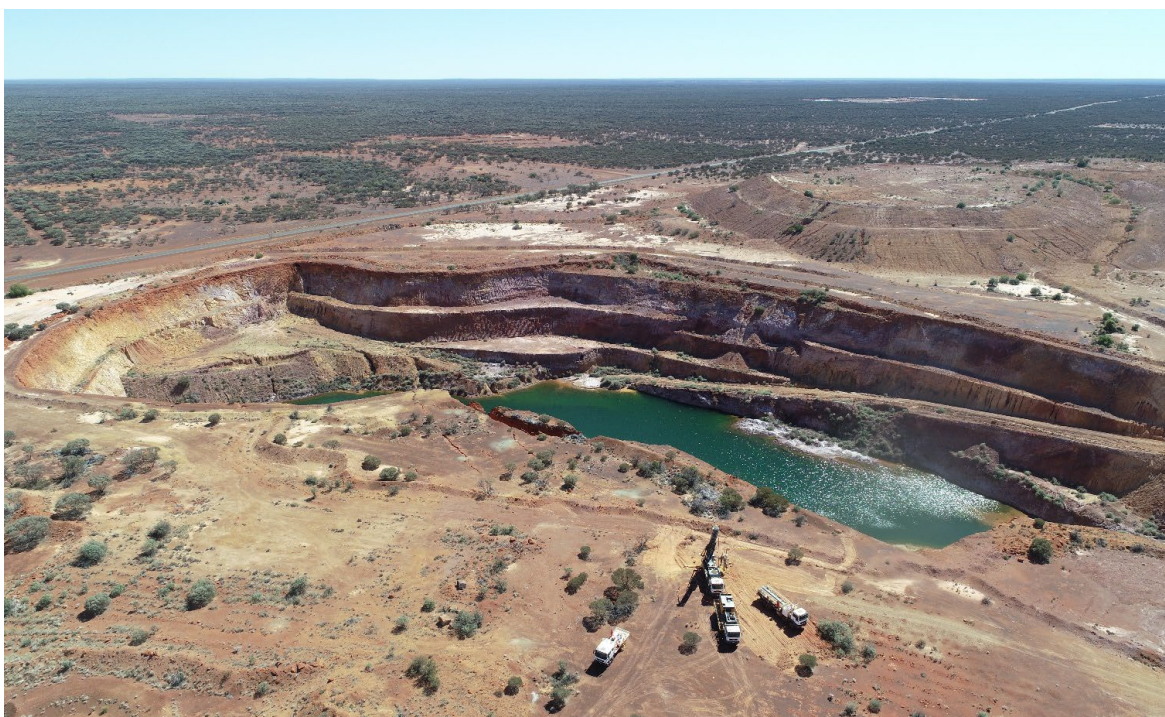
Figure 5: RC drilling underway at the historic high-grade Oroya mine, Sandstone Gold Project, WA.
