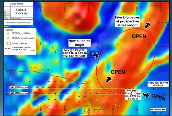
Plan map of drilling at Callisto with priority drill target zone. Red dashed lines show current mineralised interpretation at 0.5 g/t 3E cutoff projected to surface.
