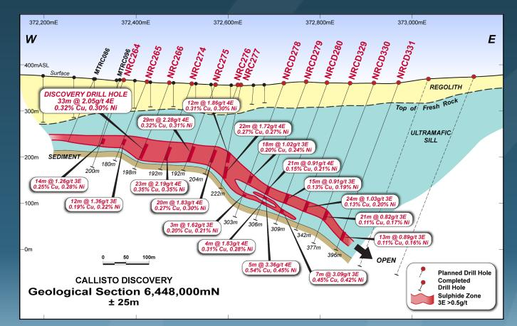
Callisto geological interpretation section 6,448,000mN with discovery drill hole NRC266. 3E = Palladium (Pd) + Platinum (Pt) + Gold (Au) in g/t
