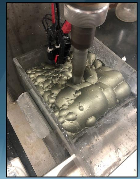
Sulphide flotation of Callisto sample from NRCD337
