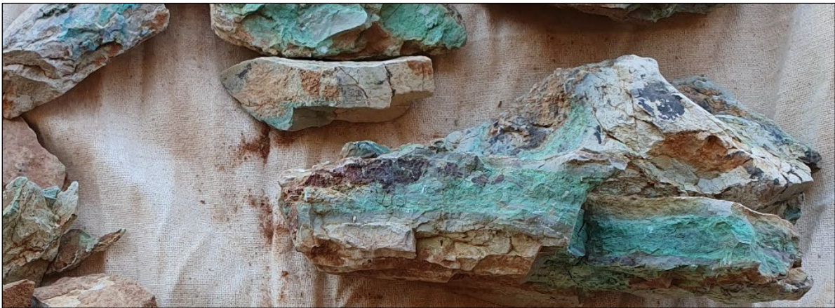
Photo 4. Rock chip sample KB03113, which returned 15.3% Copper , comprised of oxidized white meta-tuffaceous siltstone with oxide copper mineralisation (teal/green in photo).
