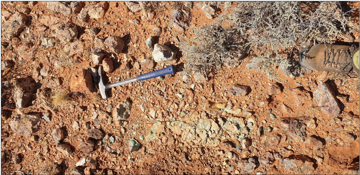
Photo 3. Photo of green malachite staining in outcrop/subcrop. Previously reported as 5.62% Copper rock chip (2019 sample KB03373).
