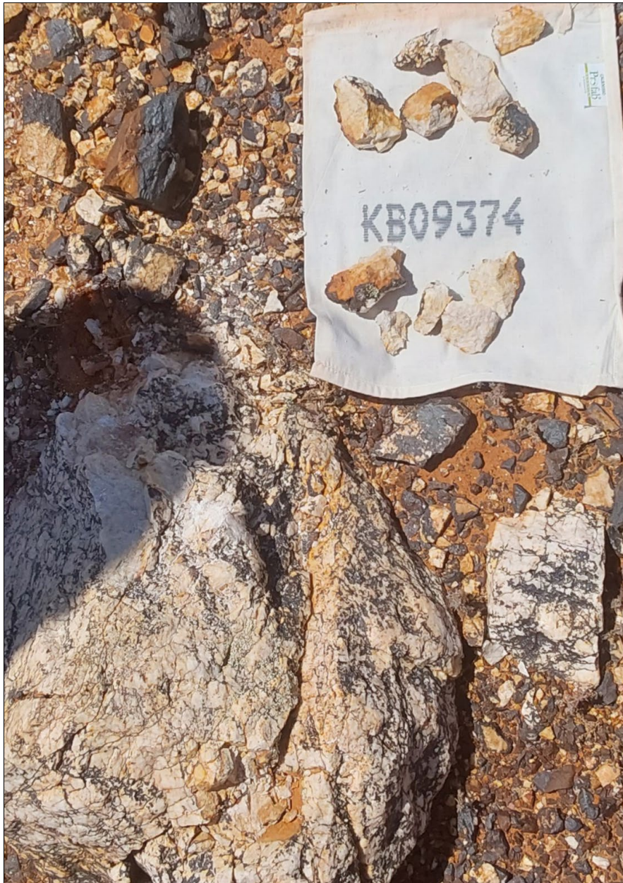
Photo 2. Quartz vein outcrop returning 22.5g/t Gold rock chip assay (KB09374); comprised of milky white and brecciated vein quartz, with iron and limonite in fractures throughout. Sample bag is 30 cm wide for scale.
