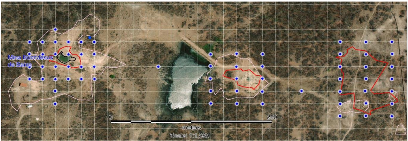
Figure 1: Google Earth image showing the 20m x 20m scout drill grids (blue dots proposed drill holes) starting in the west at the Mina Bom Jesus de Baixo pit and moving east over the other two (2) outcropping areas (red polygon being pegmatite outcrop; pink polygon being pegmatite rubble).
