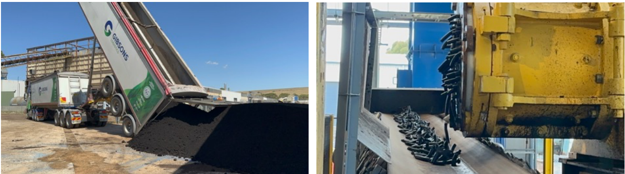
Photos (above): Receiving 40t delivery of Yallourn lignite (left) and extrusion of COLDry pellets for conditioning system trials.
