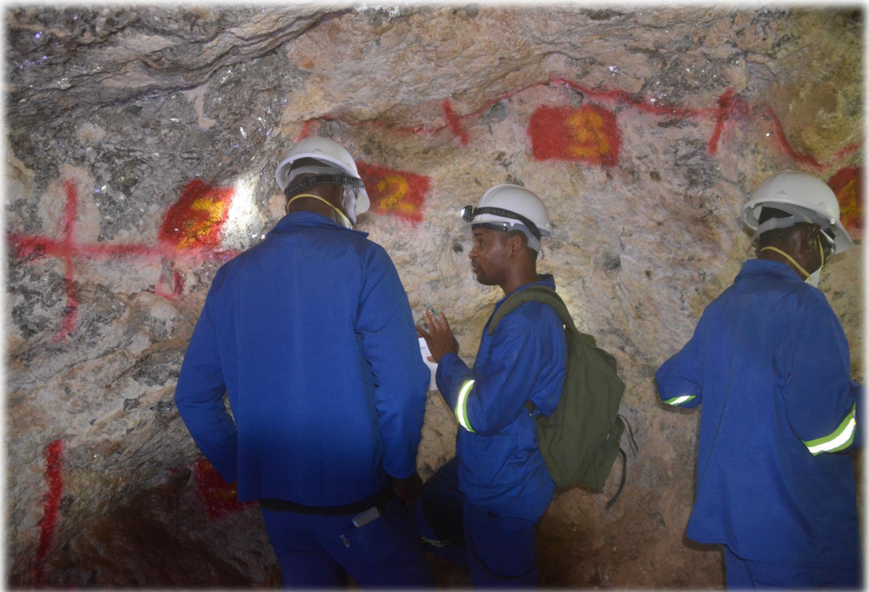
Figure 3: Prospect staff undertaking detailed underground adit sampling at Karlsbrunn
