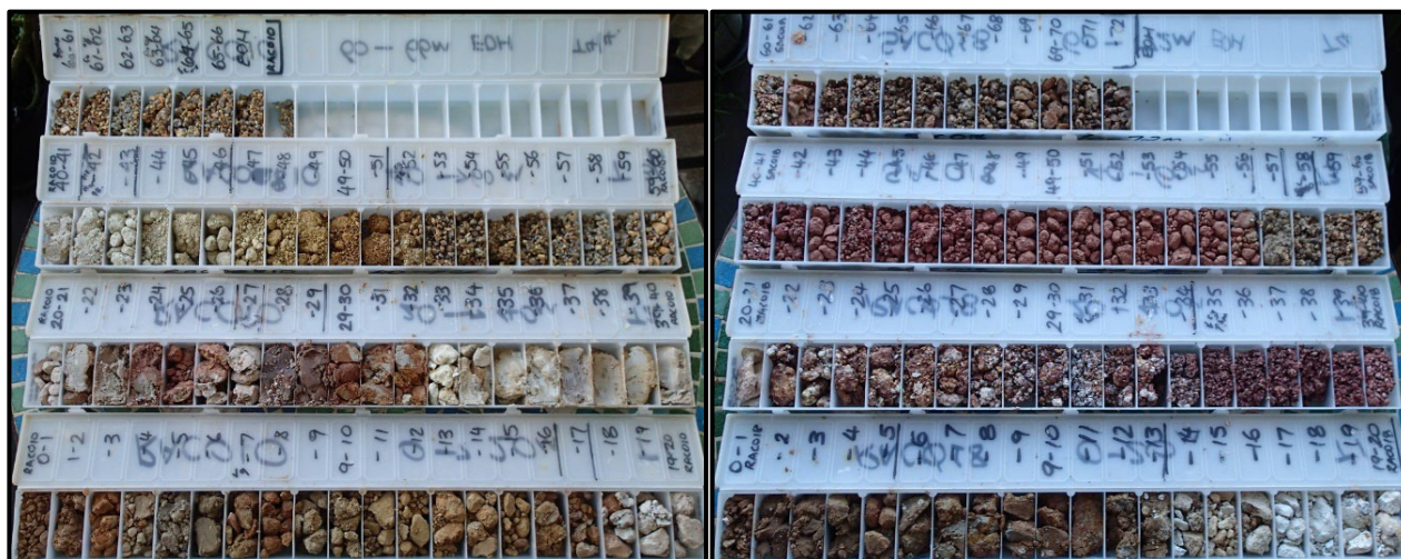
Figure 10: AC chips from RAC010 (66m TD), Ryan Granite (left); and (b) RAC018 (72m TD), Jindera Granite (right) showing red hematitic clays, yellow-orange goethitic material and white clays (pallid zones)
