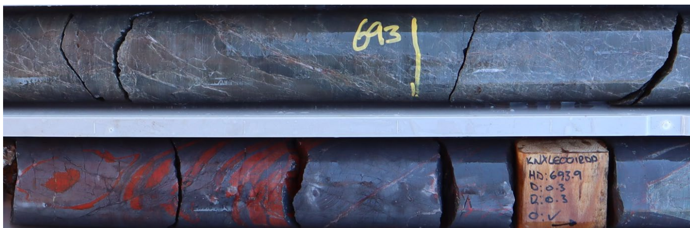
Figure 9. Ironstone that hosts 0.24% U_3O_8 mineralisation from 689.09 – 689.41m in drillhole KNXLE001RDD.
