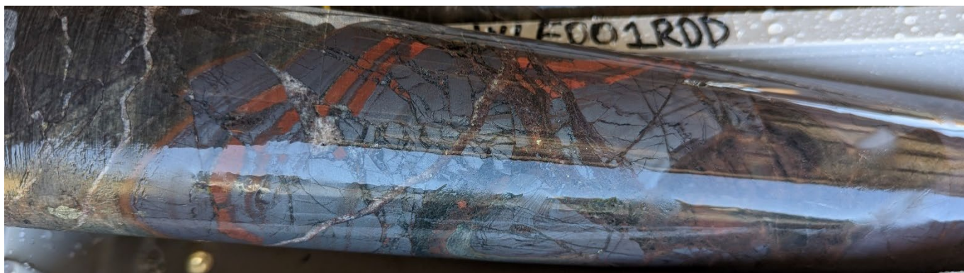
Figure 8. Ironstone that hosts 0.24% U_3O_8 mineralisation from 689.09 – 689.41m in drill-hole KNXLE001RDD.
