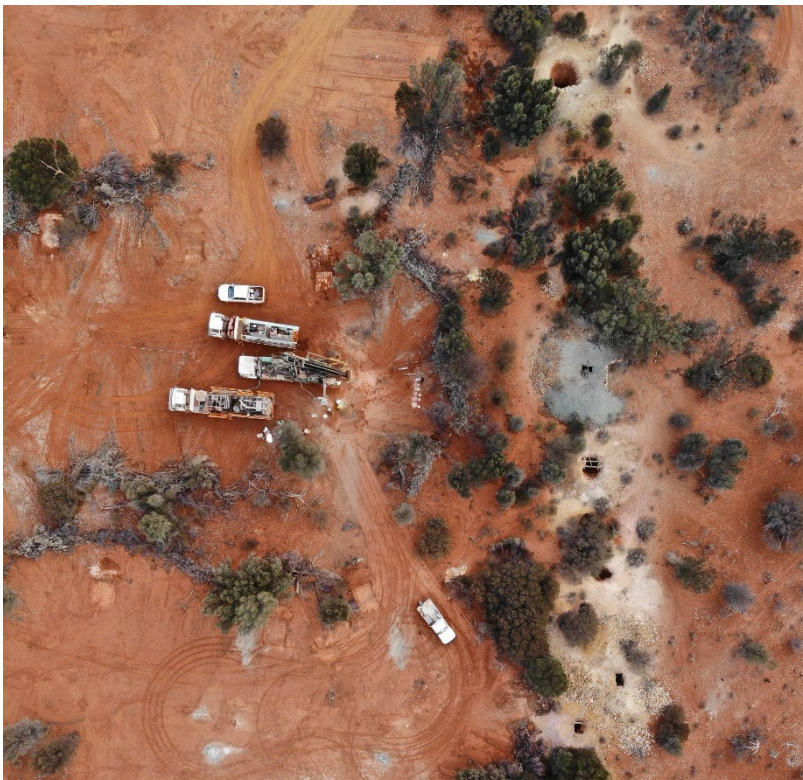
Figure 1: Drone imagery of RC drilling at Metzke’s Find with historic shallow workings seen along the line of the Metzke’s Lode.
