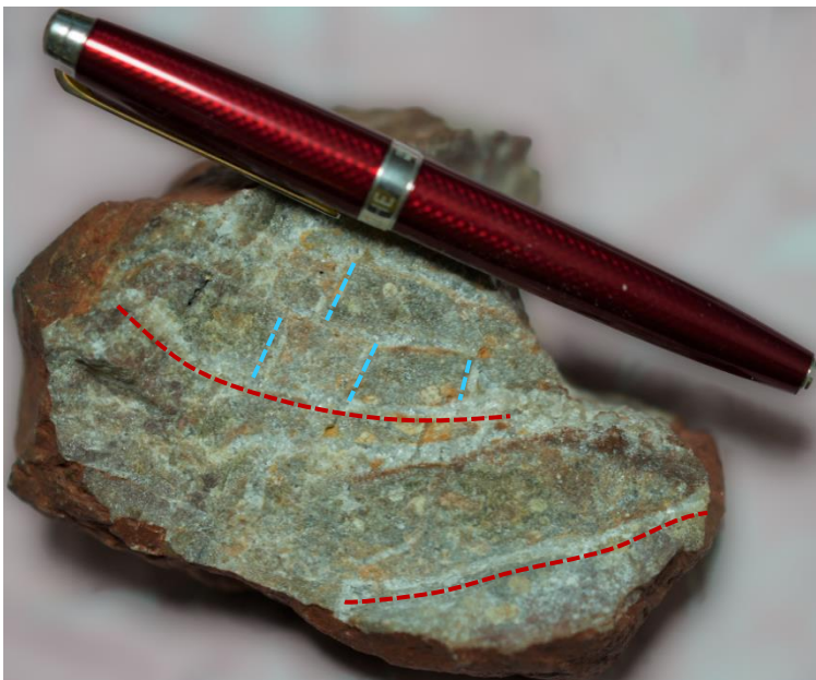
Rock chip sample from location MER1_02. Early vein sets (e.g. blue dash) and altered brecciated groundmass are enriched in molybdenum. Later vein sets (e.g. red dash) are enriched in molybdenum and silver.
