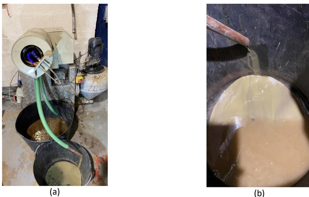
**Figure 6: (a) Testing using the Micro MGS at Gravity Mining in the United Kingdom. (b) REO concentrate product from the MGS.**
