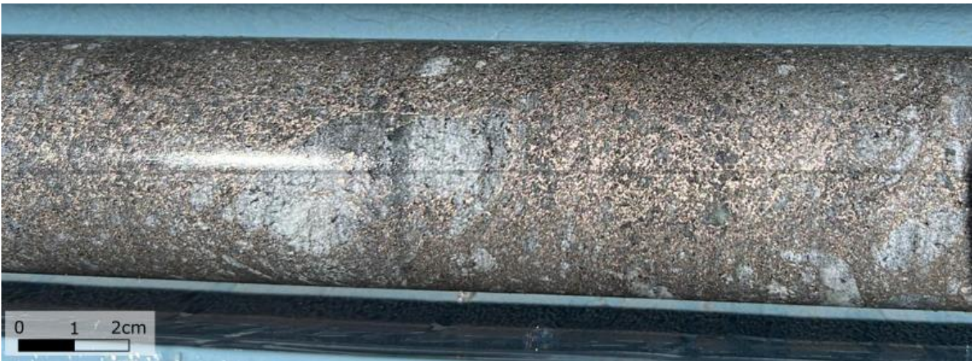
Figure 5: Photo of core from BUDD0001 showing the first sulphidic conductor returning 1.13m at 1.83g/t Ag and 0.12% Cu from 46.39m 4
