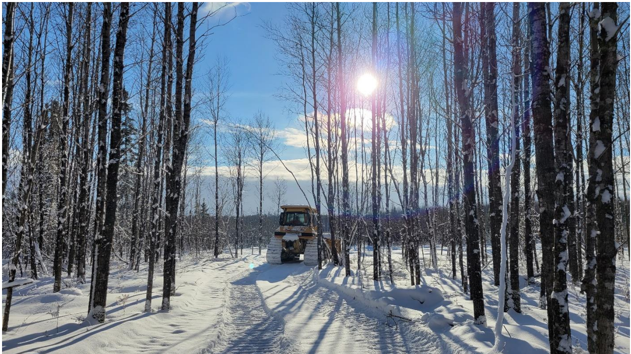
Photo 2: Dozer prepared access tracks and drill pads - Completed in March 2023
