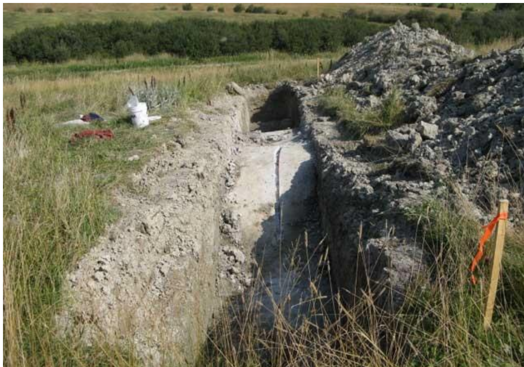
Photo 5: Bouvier Lithium Project – Trenching Cross section from 2010 Programme where the spodumene bearing pegmatite averaged 1.51% Li 2 O 13
