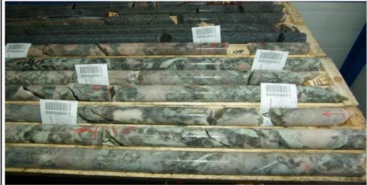
Figure 6: Core Samples from Main Dyke -showing large crystal structure of the spodumene-bearing pegmatites - 12m at 1.57% \text{Li}_2\text{O} from 108m in 21-CH-15 1
