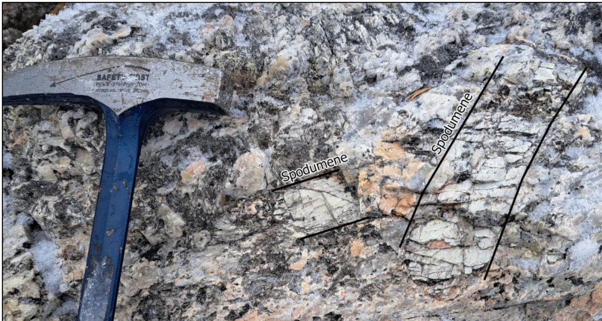
Figure 3: Coarse spodumene crystals at Greenbush 1
