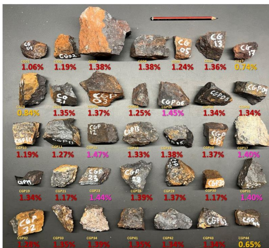
Figure 6 - Rock chip samples collected at the Canegrass Battery Minerals Project with associated analytical result for %V 2 O 5
