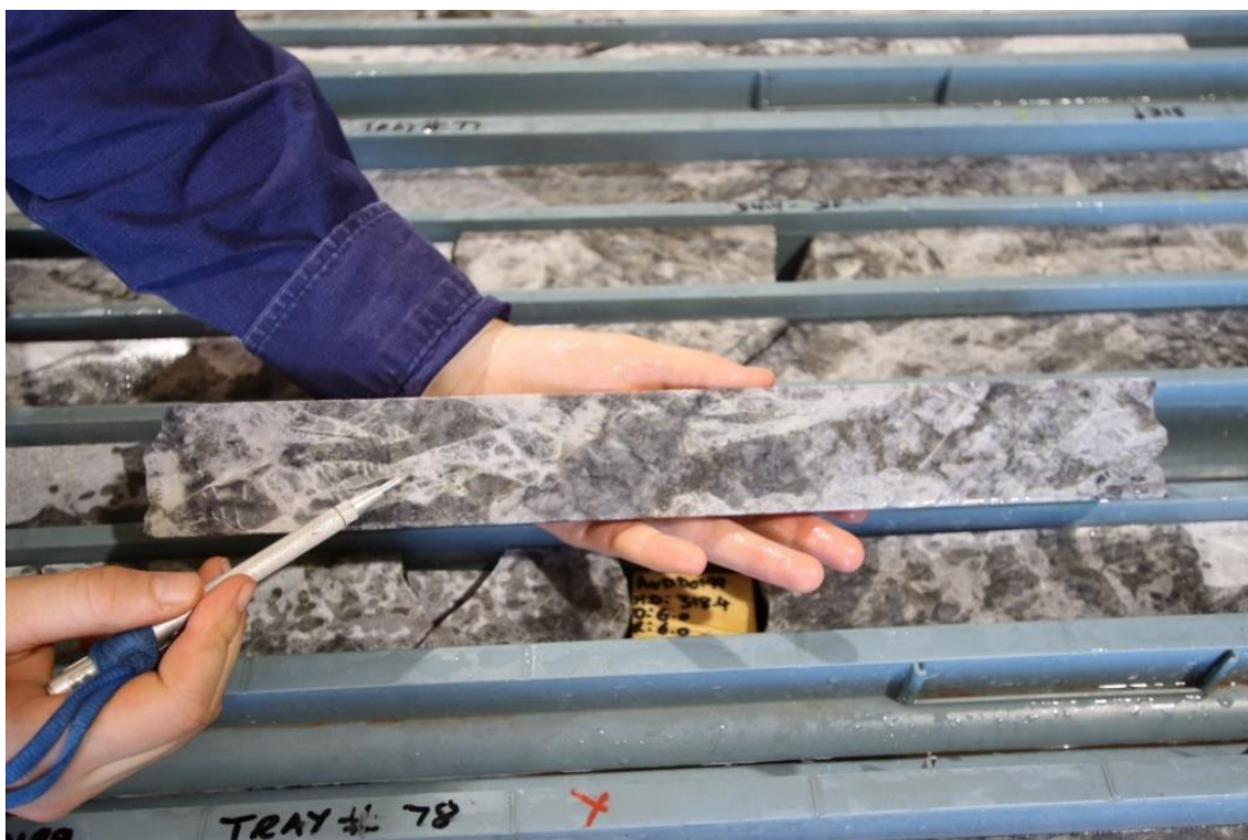
Image 1: Coarse-bladed spodumene (white crystals) in grey quartz in hole ANDD0199. This sample returned 1.0m @ 1.52% Li 2 O in an overall mineralised intersection of 7.2m @ 1.51% Li 2 O.
