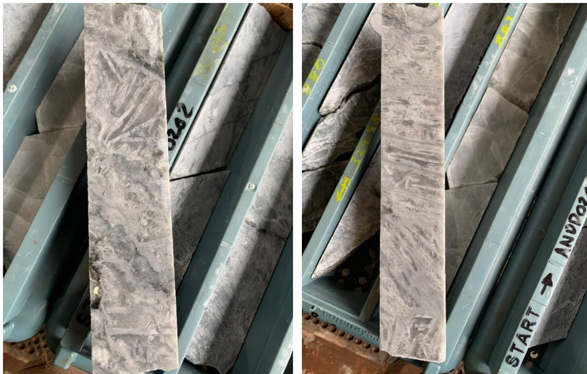
Image 2: Abundant coarse-bladed spodumene (white crystals) hosted in grey quartz matrix in pegmatite in hole ANDD0202ext at downhole depths of 333.2m (L) and 333.6m (R)
