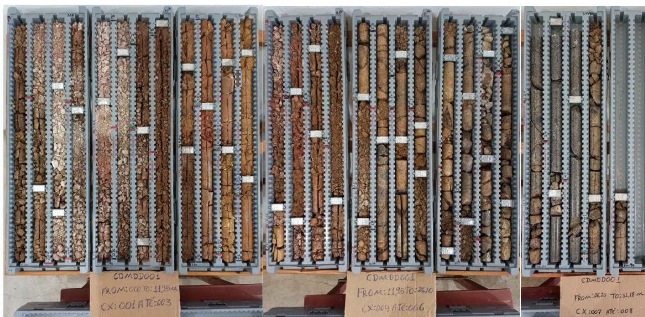
Figure 3. Core from the first diamond hole drilled at Capo Do Mel. This hole has a narrow soil horizon 0-1.4m and then a thick zone of Saprolitic clays until 26.6m. The hole finished in fresh granite at 31.8m
