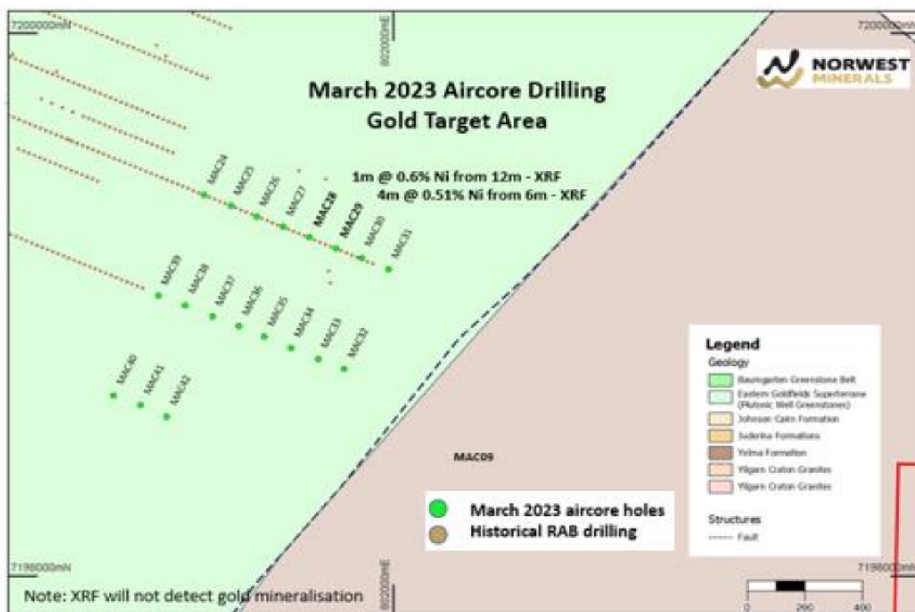
Figure 12 – Marymia East gold aircore drill targets (not detectable by XRF field analyser) – tenement E52/2395.
