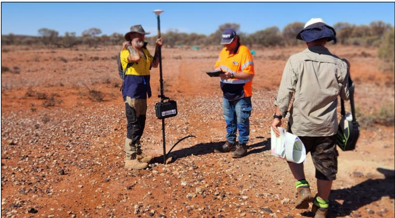
Figure 4 – DGPS surveying of drillholes at Yttria
