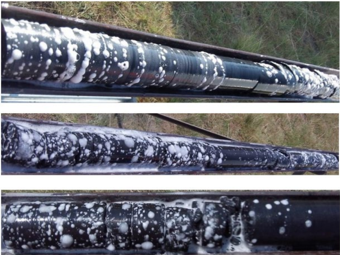
Figure 3: Core well 270-05C visible gas emissions observed from representative core samples at depths between 175-287m
