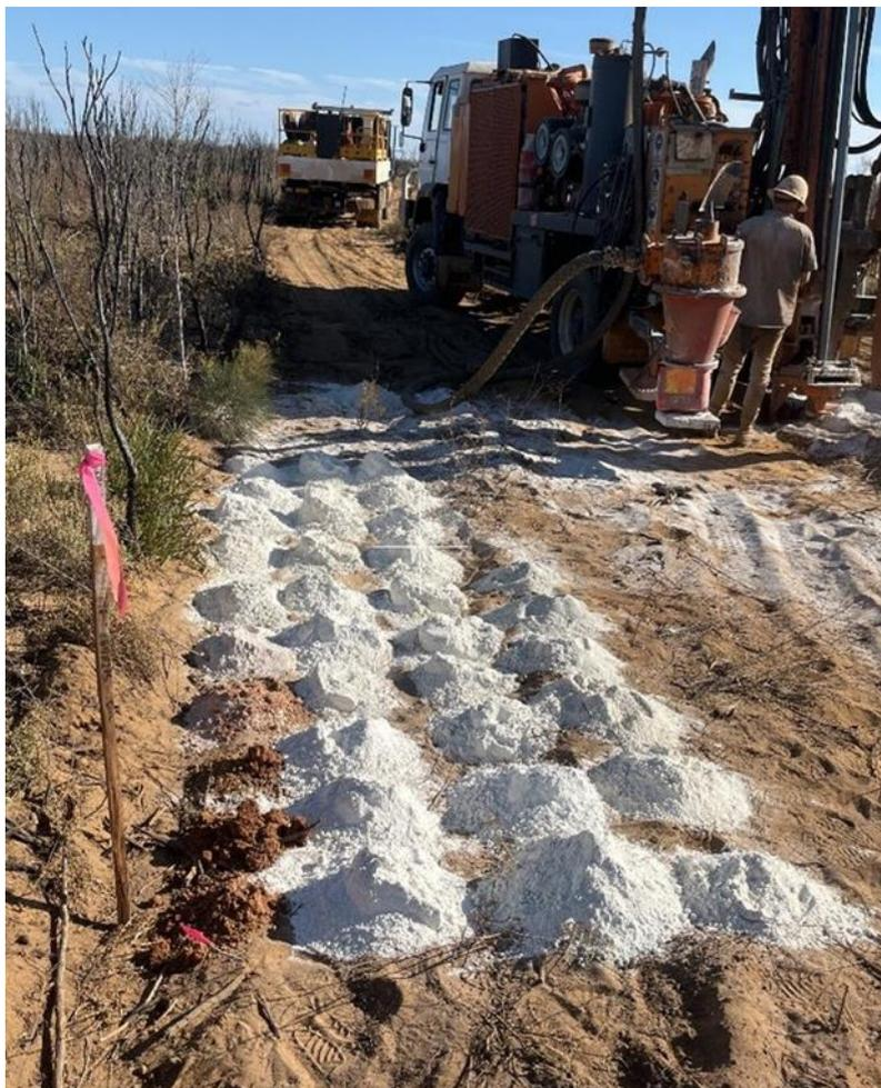
**Figure 6: High quality Kaolin intersected 30m of bright white kaolin from 4m depth (KAC014).**
