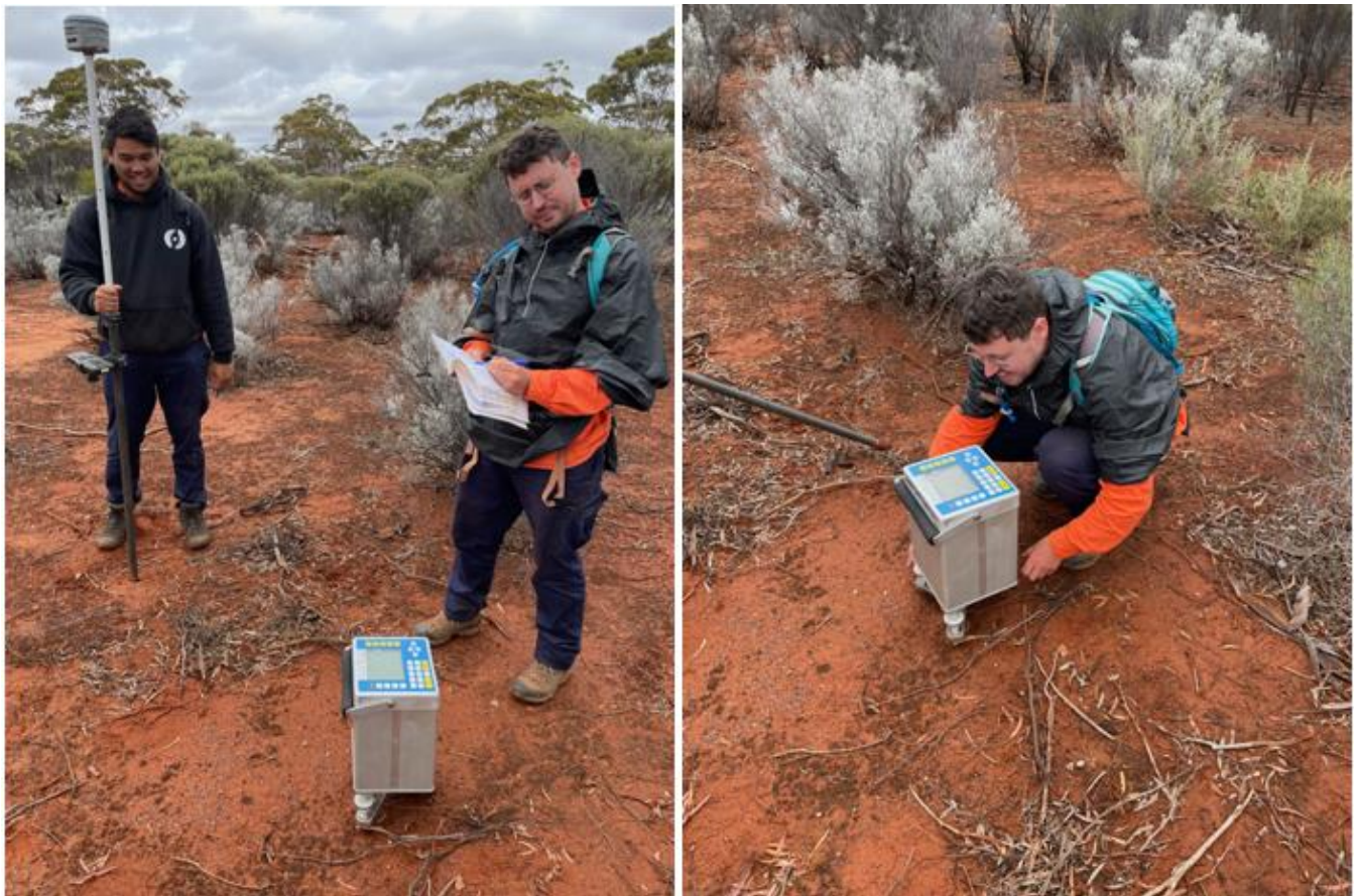
Figure 4: Technicians taking gravity readings at Hickory
