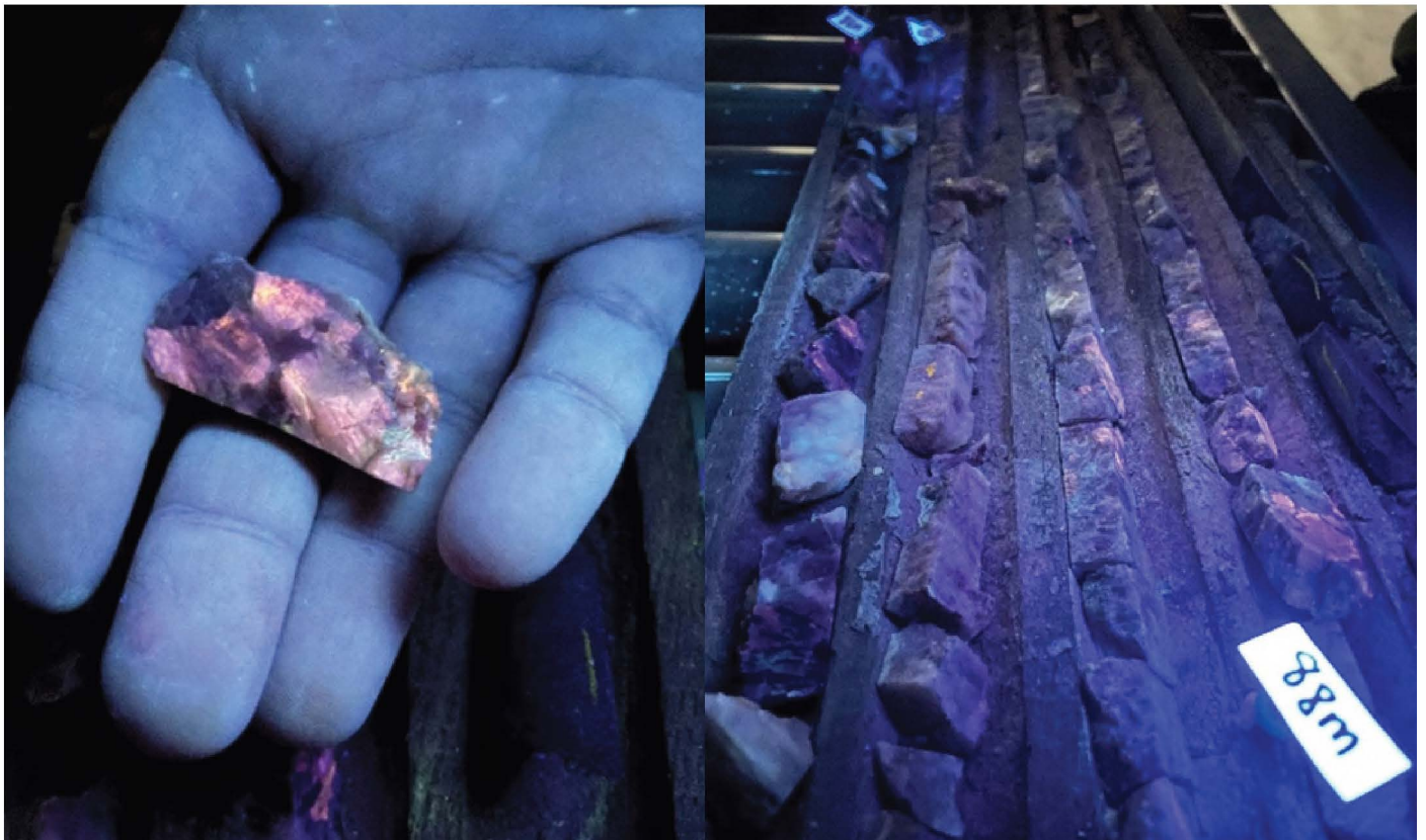
Photos of samples from XL-22 with visible Spodumene present under UV light, typically as 3-5cm crystals from interval grading 15.12m @ 1.4% Li 2 O from 73.6m. Refer ASX release 17 April 2023.
