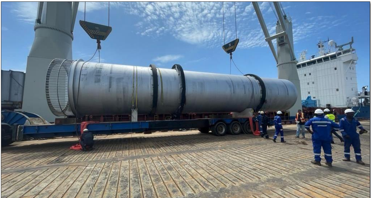
Figure 1 - Cabinda Phosphate Plant dryer being unloaded at the Port of Cabinda, Angola.
