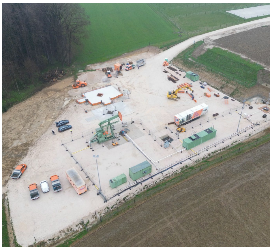
The Anshof -3 producing well and early production unit as well as the nearby concrete foundations for the Anshof-2 and Anshof-1 development wells
