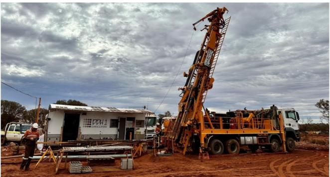
Figure 3: Convertible diamond/RC rig in the final stages of setup to commence drilling at Earaheedy.
