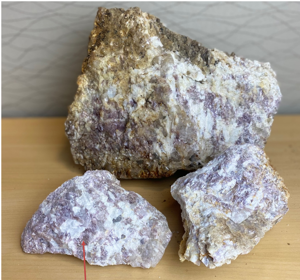
Photo: Rock samples from Pink Panther (Kanchanaburi) where LIBS analyser testing confirmed 3.45% Li (7.4% \text{Li}_2\text{O} ) in lepidolite bearing pegmatites
