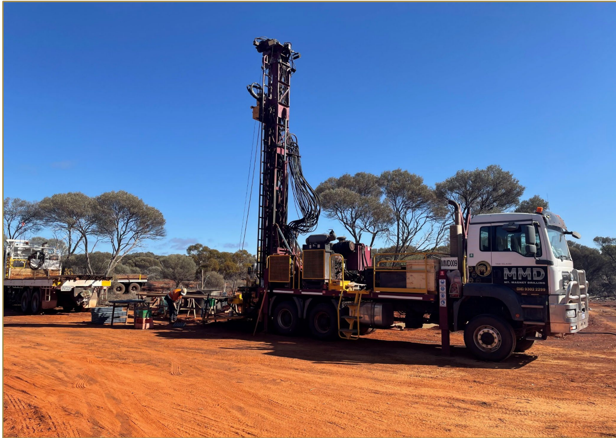
Figure 8: Diamond drill rig at the Ironstone Gold prospect
