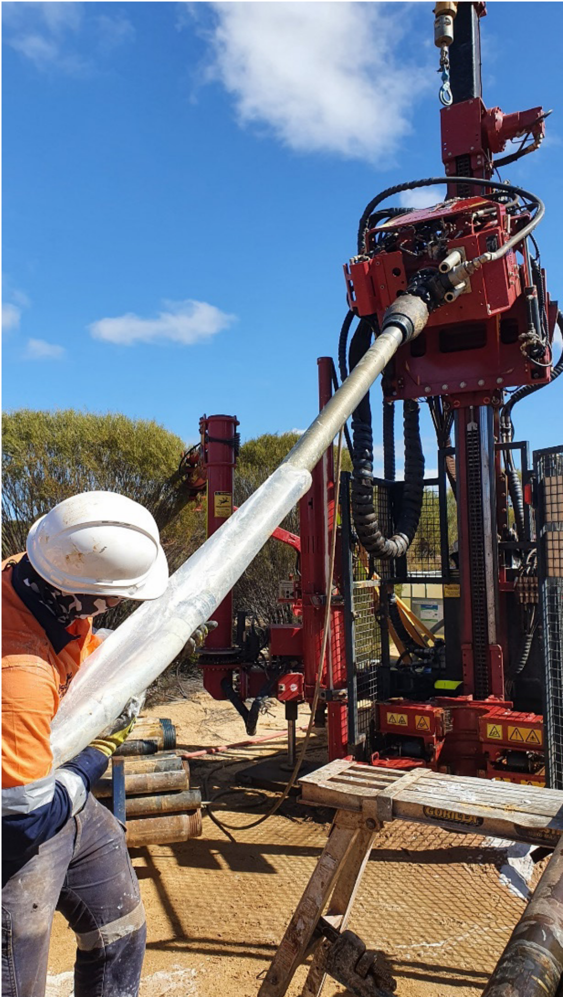
Figure 4: 2022 Resource definition sonic drilling at Tampu
